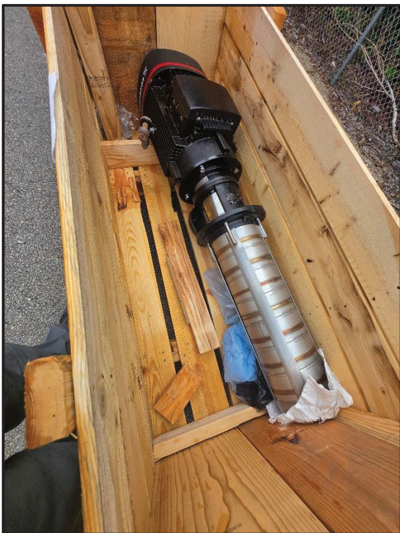
Figures 1 & 2: Cast Iron Backwash Pump & Placement
