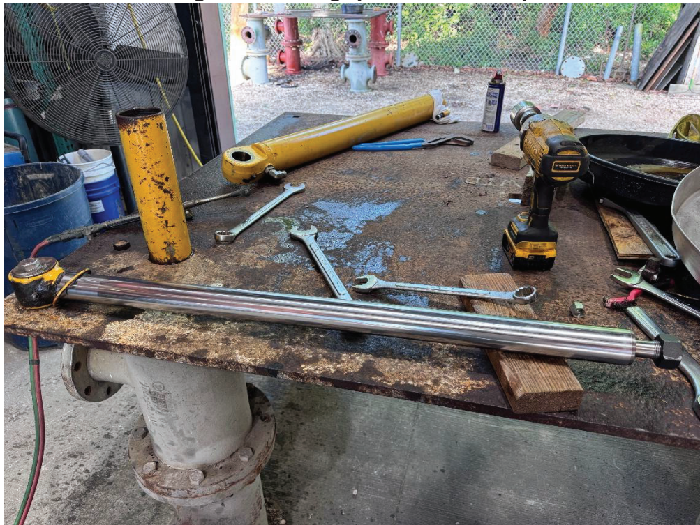
Figure 4: Loader bucket cylinder dissassembly and cleaning
