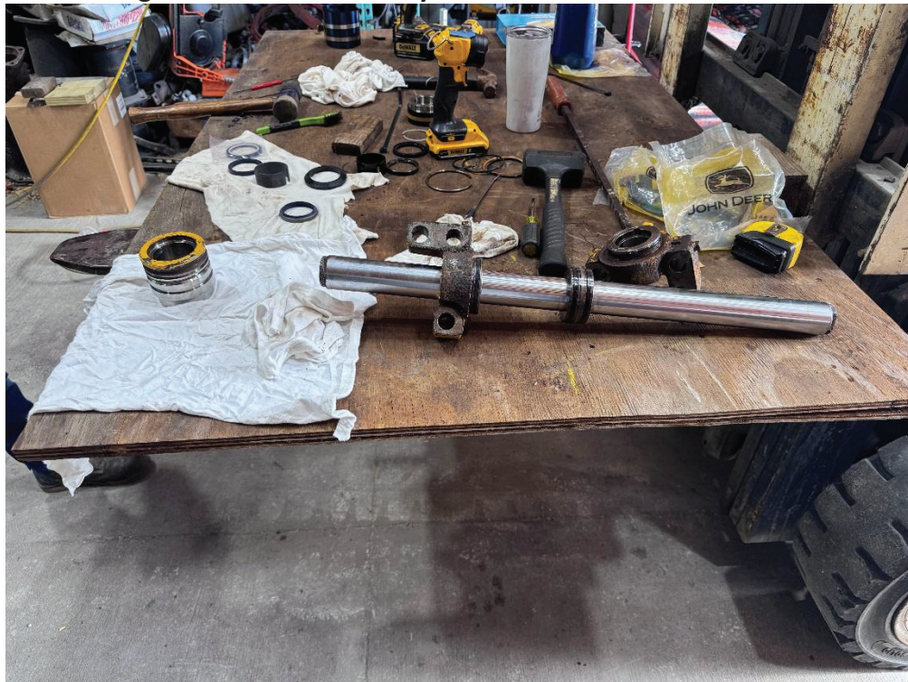
Figure 2: Steering cylinder disassembly and cleaning
