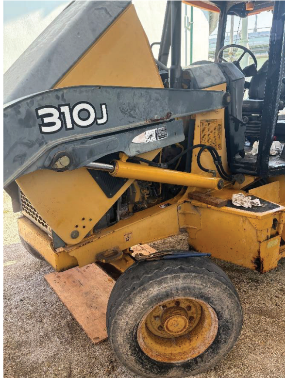
Figure 6: Rebuilt loader bucket cylinder reinstalled and tested
