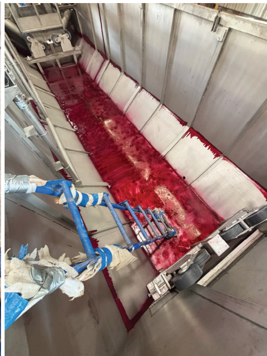
Figures 7 & 8. Filtration Upgrades CWI Dye Penetration Testing
