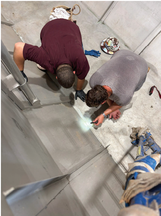
Figures 7 & 8. Filtration Upgrades CWI Dye Penetration Testing
