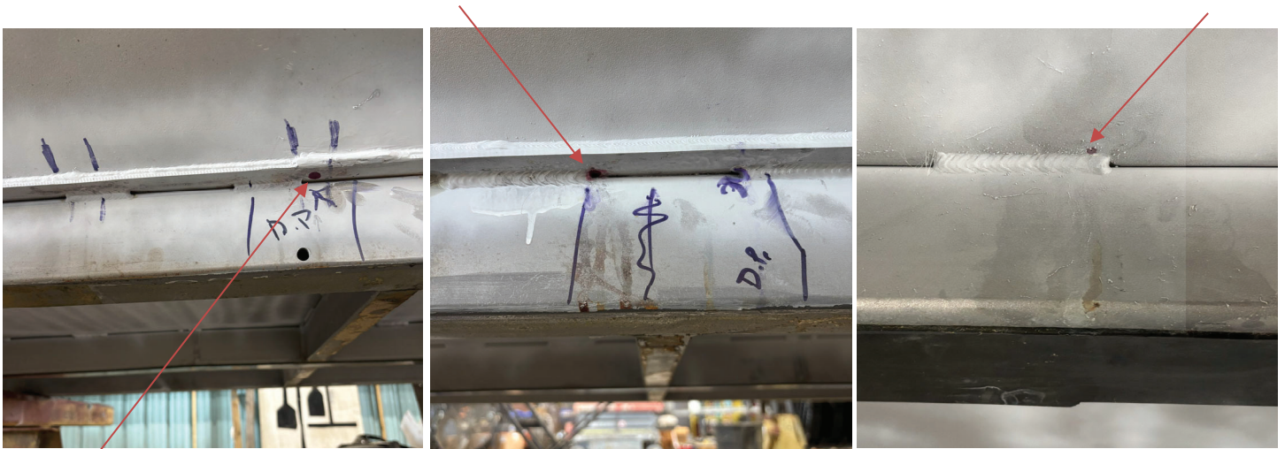
Figures 9 & 10. Filtration Upgrades CWI Dye Penetration Testing
