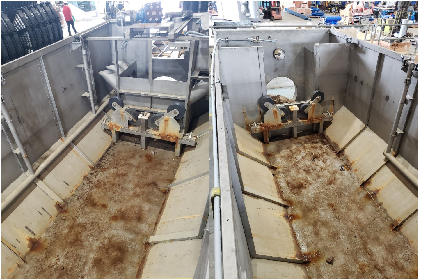
Figure 6 and 7. Corrosion on the 316SS Evoqua 40X filter (At Evoqua Factory).
