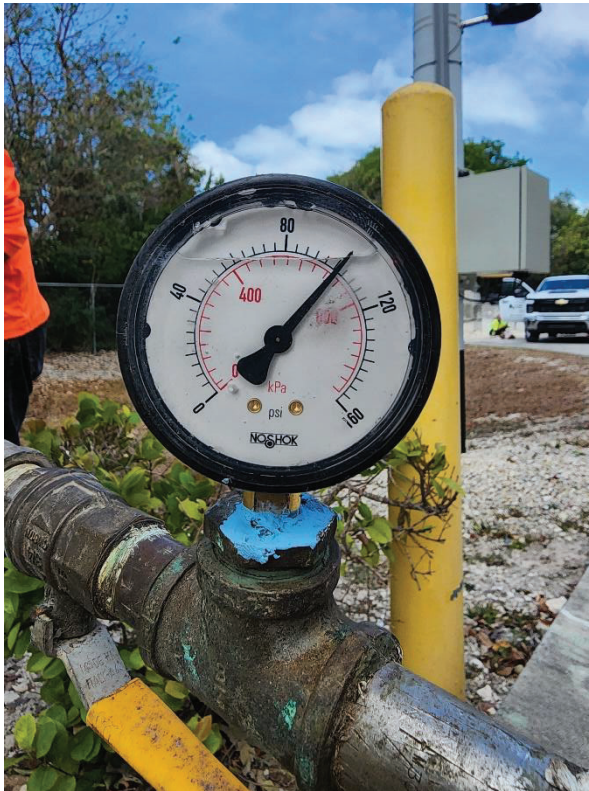
Figure 16 and 17. Pressure testing of force main piping for the VPS job at Vacuum Station D
