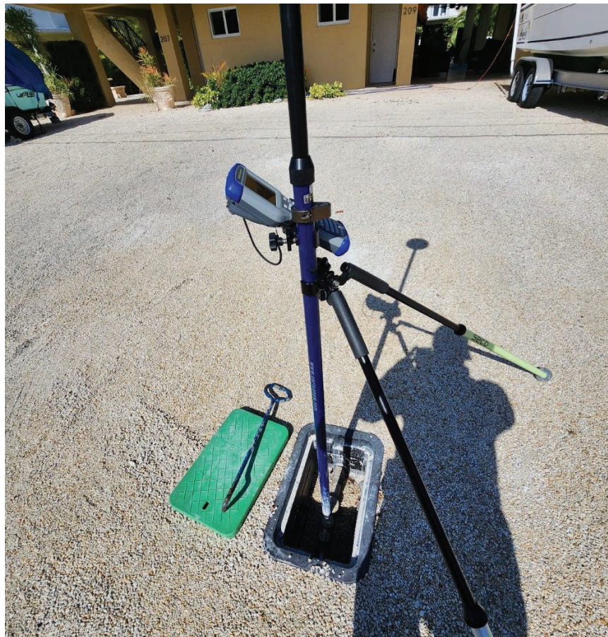
Figure 9. GPSing elevations and locations of all valves
