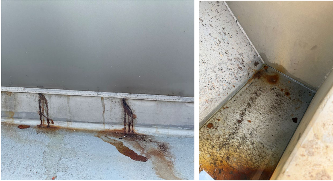
Figure 4 and 5. Corrosion on the 316SS Evoqua 40X filter (On Site).
