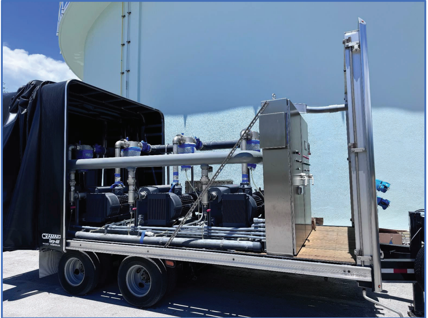
Figure 1: Emergency vacuum trailer side view.
