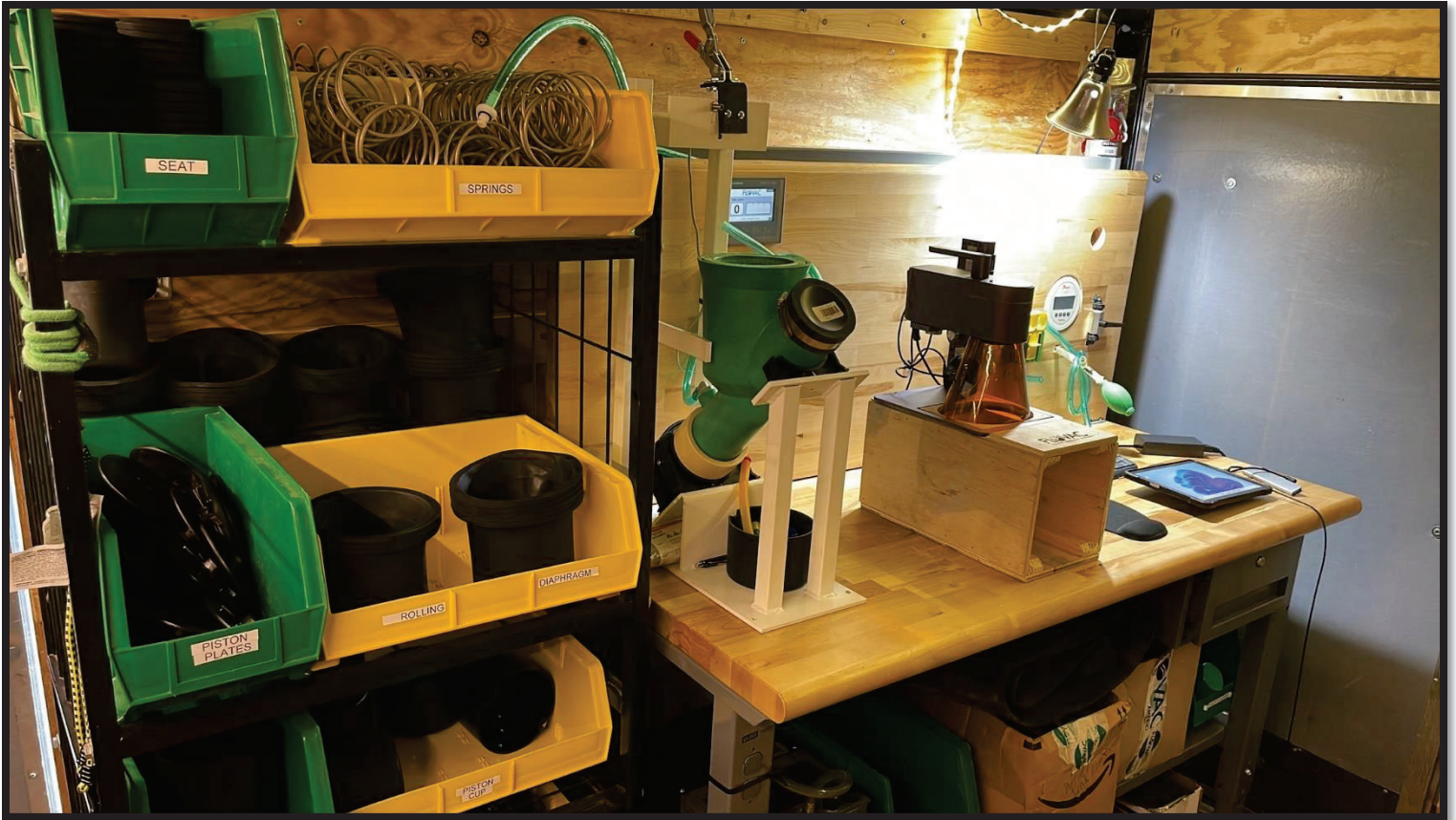
Figure 7: Work station inside of the Flovac Valve Rebuild Trailer
