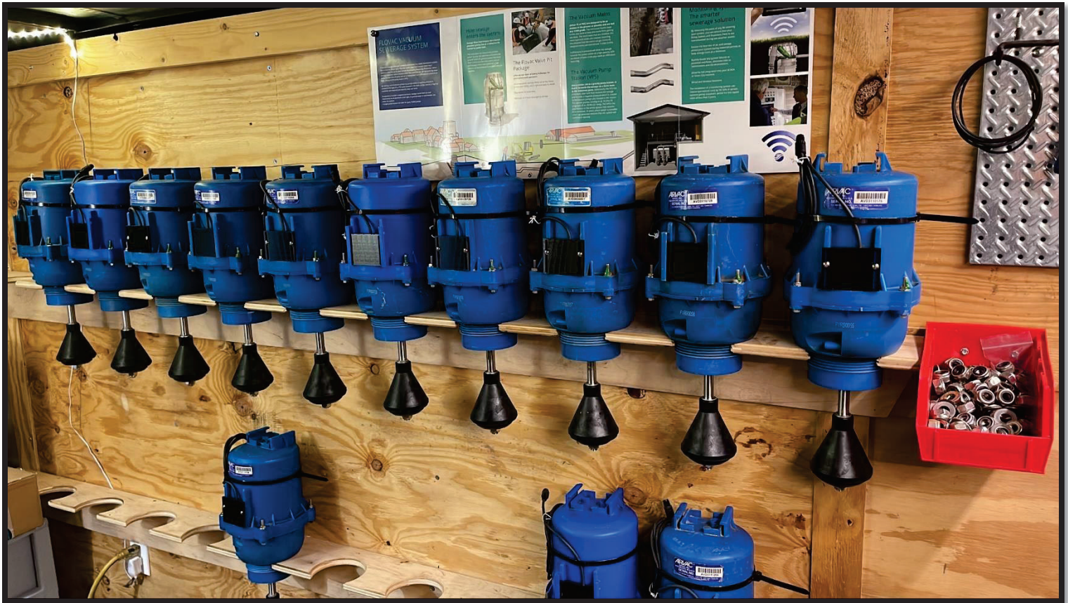
Figure 8: KLWTD Vacuum Monitoring Rebuilt Valves
