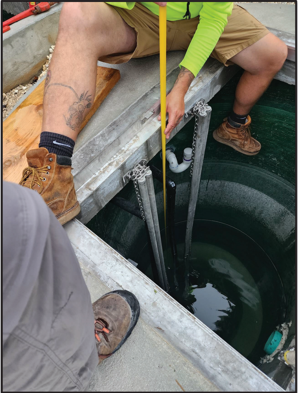
Figure 8: Water Level Checked Prior to Draw Down Testing, and Between Each Test by F.J. Nugent
