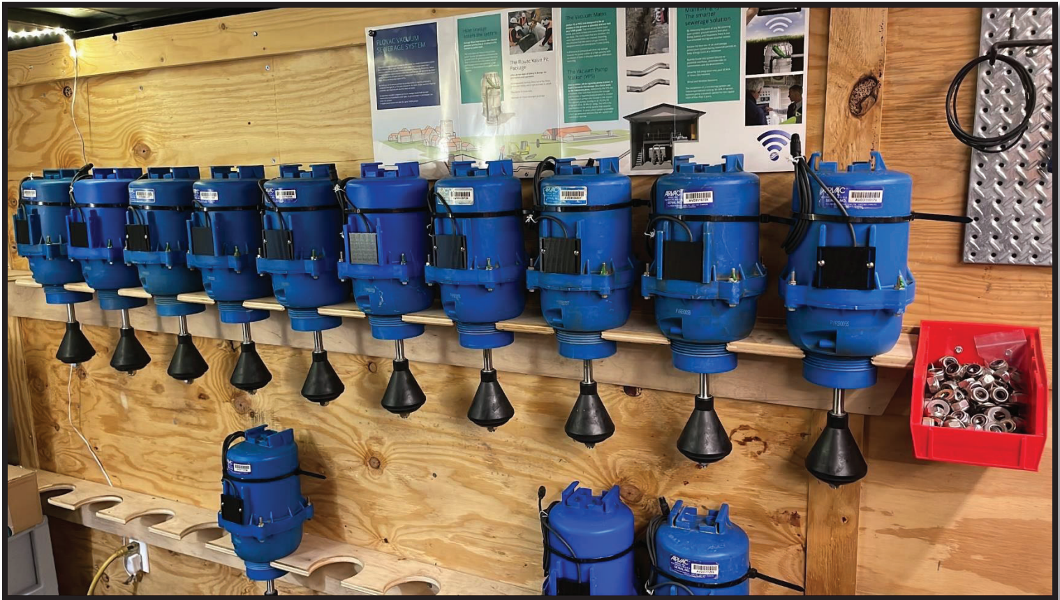
Figure 8: KLWTD Vacuum Monitoring Rebuilt Valves
