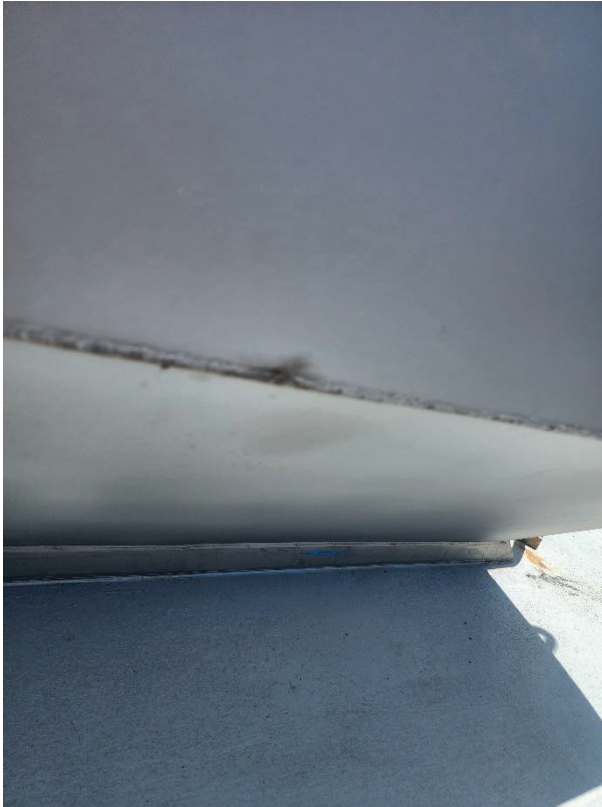
Figure 4 and 5. Corrosion on the welds of the 316SS Evoqua 40X filter
